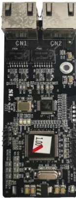
Ethernet/IP communication card EC-TX510/ EC-TX515
